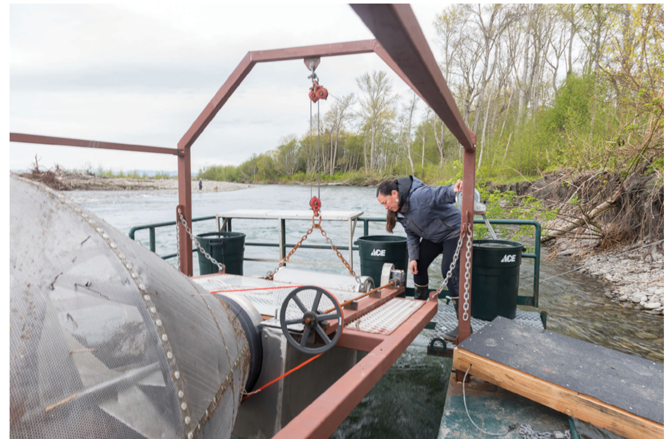
Above: Vanessa Castle checks the mechanics of a rotary screw trap, which traps migrating fish in an underwater holding tank, where they can then be counted and measured before release.
